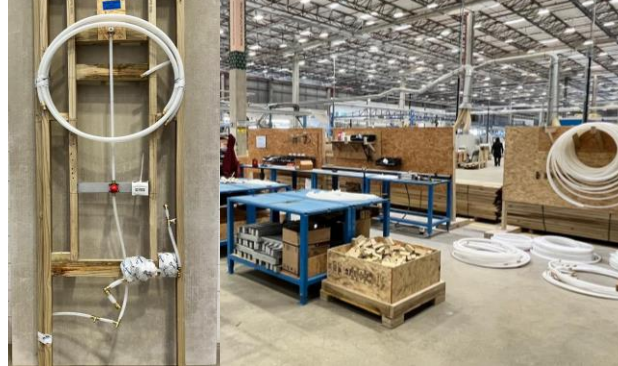
2. Shaft assembly station and hydraulic kit
